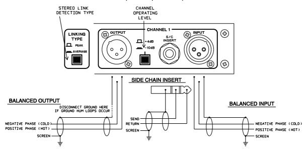
FOR UNBALANCED OPERATION, CONNECT NEGATIVE PHASES TO GROUND AT INPUT AND OUTPUT
