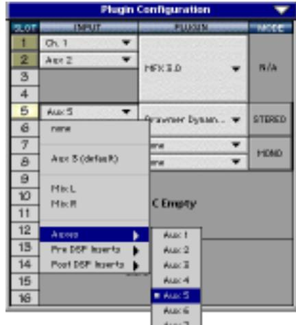
A plug-in can also receive its input from a channel pre- or post-DSP insert or the main stereo left and right Bus insert. When a plug-in is inserted “in line” in this manner, its output is routed directly back into the channel. See “FX Routing” on page 26 for more details, especially in regards to stereo routing.
