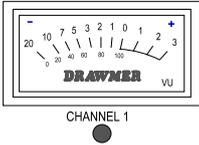
A moving coil VU meter monitors either the level of the output signal (over the range -10dB to +10dB with reference to the +4dBu operating level) or the amount of gain reduction taking place. Because the meter has VU characteristics, it closely reflects what is actually being heard, though will not respond quickly enough to register short signal peaks.
