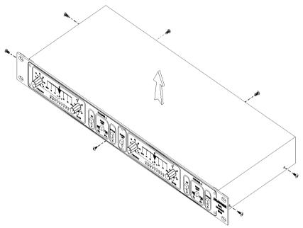
Removing seven screws to access internal fuse
