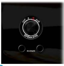
main outputs (A) (B) when plugged in, whilst the left socket leaves the outputs as is - though this can be altered via the internal jumper settings (see 'Internal Jumpers Settings').
