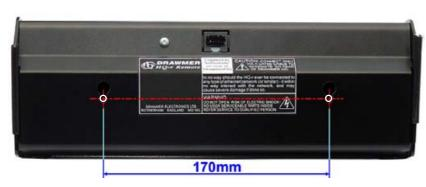
The remote can be fixed to a desk to provide further stability via the the two holes on the bottom of the unit. Screw in to a desk two screws at a distance of 170mm apart and to a depth of 5mm to the shoulder, then slot the
