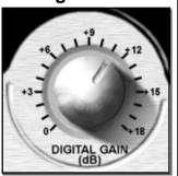
GAIN of up to +18dB can be applied. Be aware that digital distortion can occur
