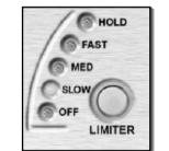
The limiter will only have any effect when 'DIGITAL GAIN' is set greater than 0dB.
