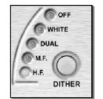
H.F dither generally removes the low level distortion on low signal levels with the least noticable noise.
