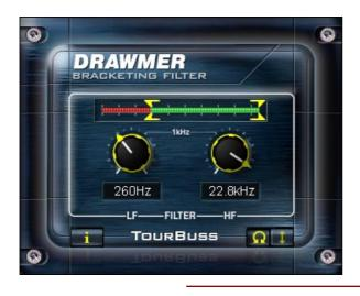
A Bracketing Filter has been incorporated in to the TourBuss suite, providing Low and High 12dB per octave filters that attenuate any unwanted frequencies. Thus making it simple to remove unwanted frequencies without using the resources that a more complicated equaliser would utilise.
