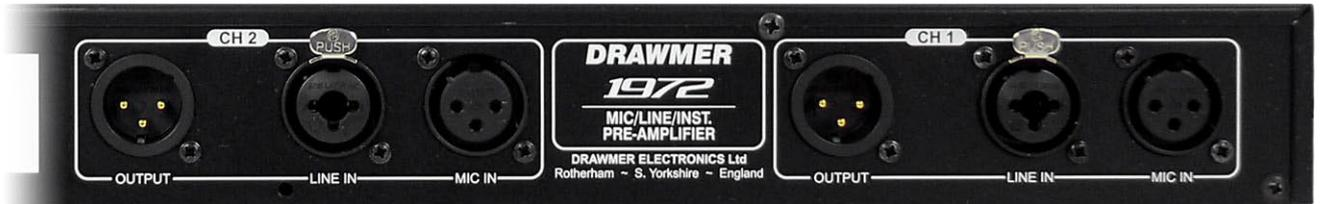
In addition to the instrument input 1/4" jack connector located in the instrument section on the front panel there are also several found on the rear panel:
