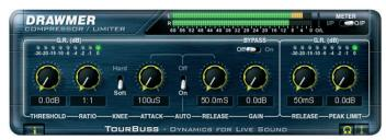
The Tourbuss Compressor combines aspects of both the traditional ratio style compressor and the soft knee approach, making it equally adept at creative work and unobtrusive level control. Many advanced facilities that enable quick setup, predictable results and a musical analogue style response have been incorporated, including:
