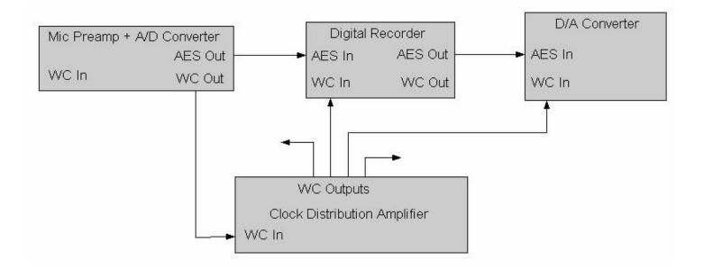
The distribution amplifier buffers the clock source and provides multiple outputs to the other devices in the system.
